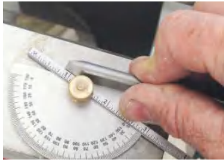
▲ Pic.5 The tool is ground to an angle of around 20°; this will allow the tool to easily slice through the fibres of the timber
